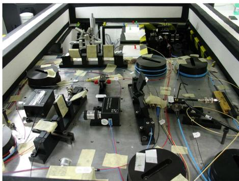
FIG. 2: Part of the experimental setup for post-selection reduction of noise thermally isolated in a polystyren box.
