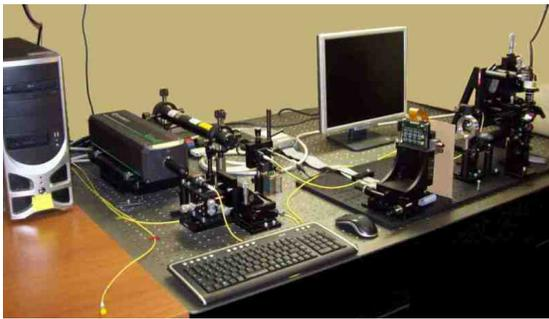
FIG. 1: Snapshot of the holographical laser tweezer.
