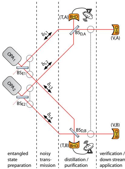
FIG. 1: Scheme for entanglement distillation of phase-diffused two-mode squeezed states.
