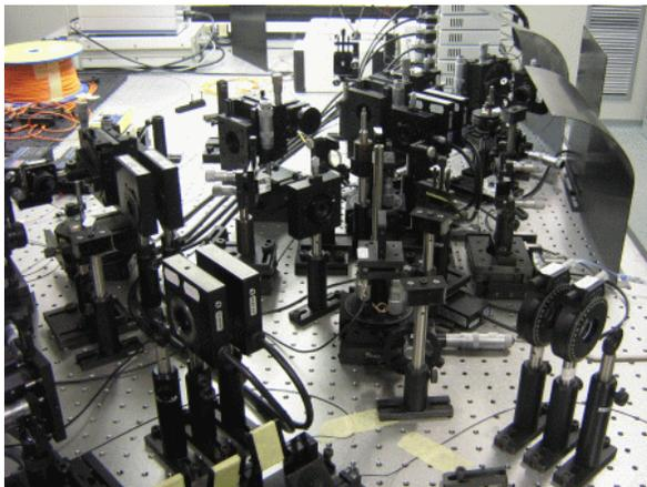
Obrázek 1: Picture of the key part of the universal quantum filter.
