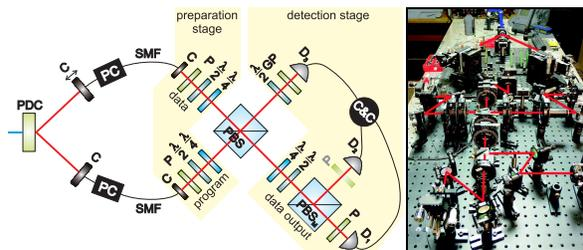
FIG. 1: Scheme of the experimental setup.
