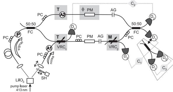
FIG. 3: Scheme of the setup for post-selection reduction of noise.
