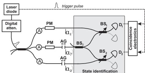
FIG. 1: Scheme of the setup for unambiguous discrimination of coherent states.
