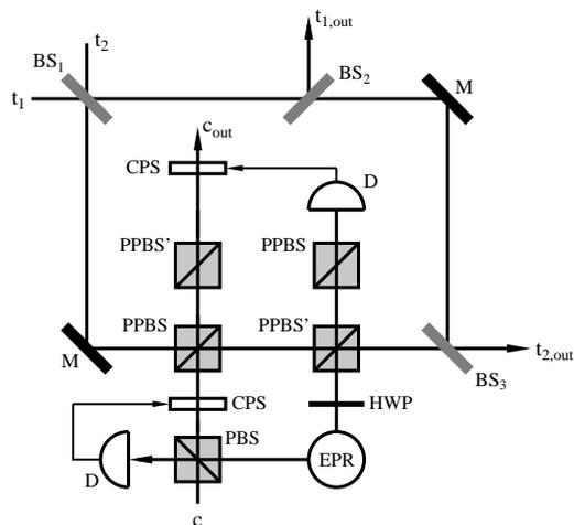
FIG. 2: Linear optical Fredkin gate operating in the coincidence basis.
