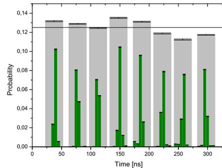
FIG. 2: Measured response function of the developed detector to weak coherent light pulses with Poissonian statistics with mean photon number of one photon per pulse at the input port of the detector. The eight distinct well-separated detection channels (light gray) are apparent in time-of-flight data. The detection probabilities of the particular channel span several 5 ns time-bins (green) due to the time uncertainty of the time-of-flight spectrometer and the source-detector jitter.
