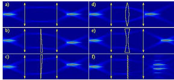
FIG. 3: Illustration of the beam shaping based on modulation of the spatial spectrum. (a) without modulation, (b) and (c) linear phase modulation (transverse relocation of the beam spot), (d) and (e) quadratic phase modulation (longitudinal relocation of the beam trail), (f) binary phase modulation (splitting of the input beam).
