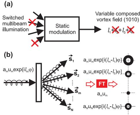
FIG. 1: Principle of the information encoding (a) and decoding (b).
