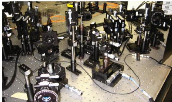
FIG. 2: Picture of the key part of the partial-SWAP quantum gate.
