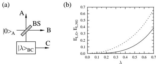
FIG. 2: (a) Scheme for preparation of a three-mode Gaussian state. (b) Maximum logarithmic negativity  $E_{L,G}$  (solid curve) for optimal Gaussian measurement on mode  $C$  and average entropy of entanglement  $E_{L,NG}$  (dashed curve) for measurement of photon number on mode  $C$  versus squeezing parameter  $\lambda$ .
