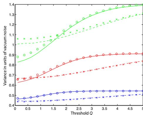
FIG. 2: Dependence of the squeezed-quadrature variance of the purified beam on the trigger threshold. Colors indicate three different levels of phase noise. Solid (dashed) lines correspond to triggering on measurements of squeezed (anti-squeezed) quadrature.
