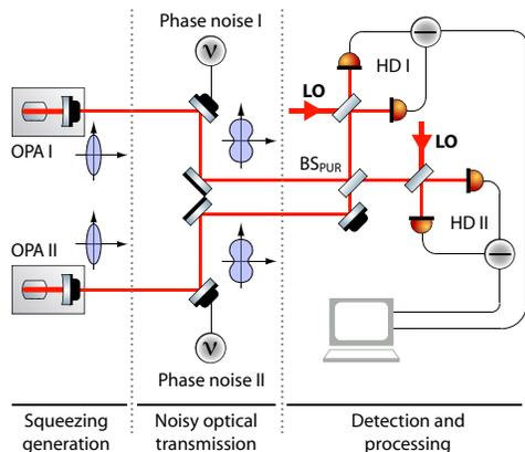
FIG. 1: Setup for purification of phase diffused squeezed beams. OPA - optical parametric oscillators, LO - local oscillator beams, HD - homodyne detectors, BS - balanced beam splitter.
