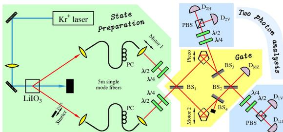
FIG. 1: Scheme of the partial-SWAP quantum gate.
