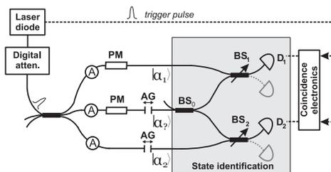
FIG. 2: Scheme of the setup for unambiguous discrimination of coherent states.
