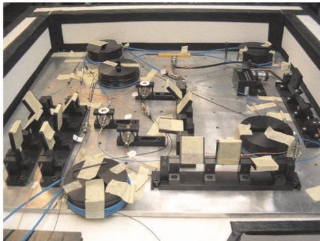
FIG. 1: Part of the experimental setup for phase-covariant quantum cloning thermally isolated in a polystyrene box.
