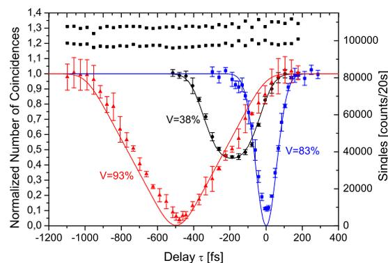
FIG. 2: The normalized number of coincidences and singles as a function of the time delay  $\tau$  in a HOM interferometer. Black dot - no pulse-front tilt, red triangle - frequency-correlated photons, blue box - frequency-anticorrelated photons, black box - single counts, solid lines - theoretical prediction.
