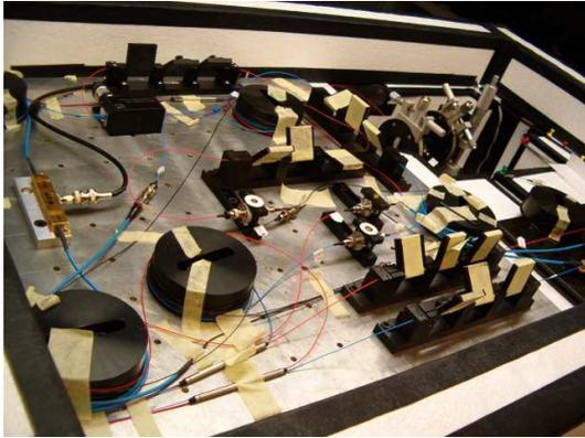
FIG. 1: Part of the experimental setup with the shielded Mach-Zehnder interferometer.
