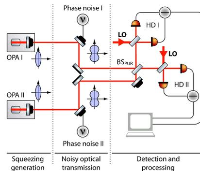
FIG. 2: Distillation of phase-diffused squeezed states.
