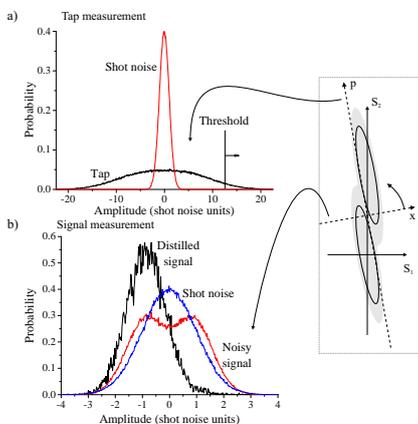
FIG. 1: Distillation of randomly displaced squeezed states.
