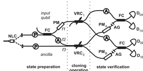
FIG. 2: Scheme of the asymmetric-cloning setup.
