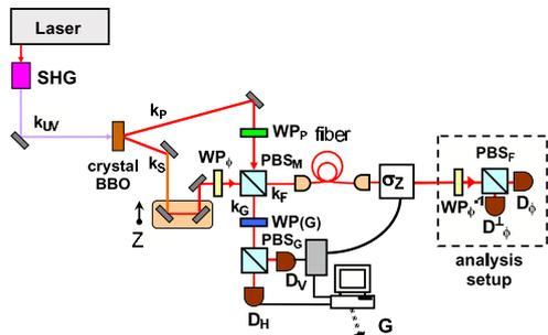
FIG. 1: Optical set-up implementing the MDM. The output qubit is characterized adopting the analysis setup illustrated in the dashed box.
