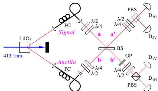
FIG. 2: Scheme of the cloning setup.
