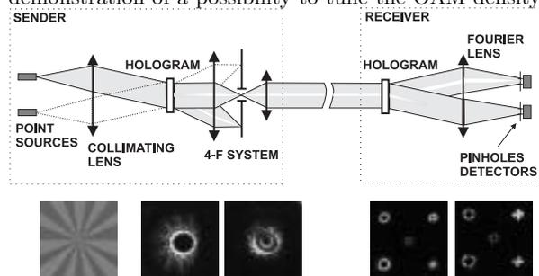
FIG. 1: Optical set up for transfer of information by means of composed vortex beams.
