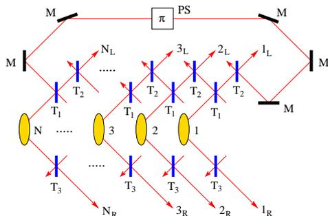
FIG. 1: Scheme for N-qubit Toffoli gate in coincidence basis.
