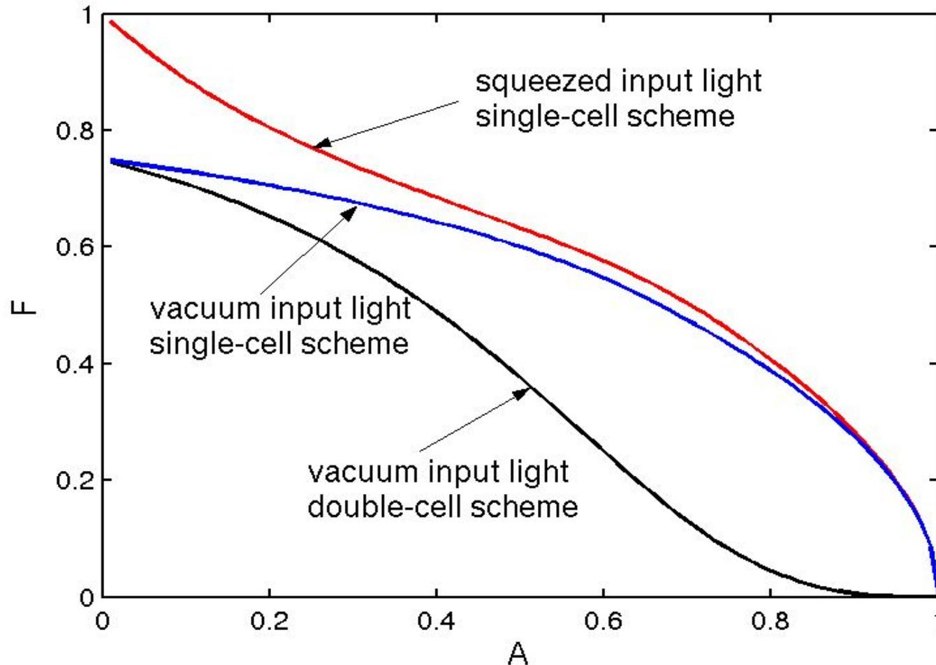
Fidelity is reduced due to losses of light on the walls of the glass cells holding the atoms.
