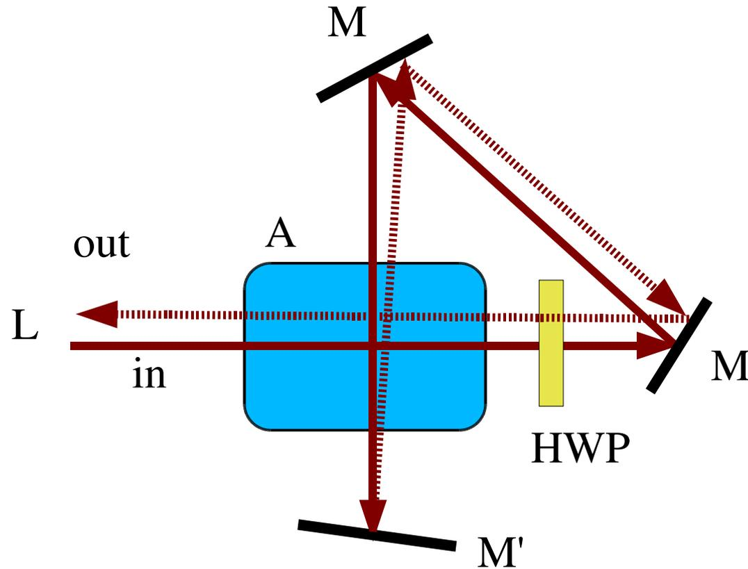
After the first two passages the light beam is reflected back and again passes twice through the atomic ensemble.
