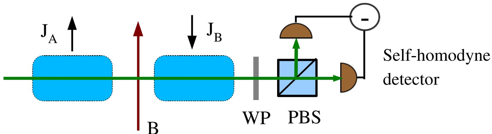
The QND interaction is recovered, a non-local atomic mode couples to the  $\cos(\Omega t)$  mode of the light beam.
