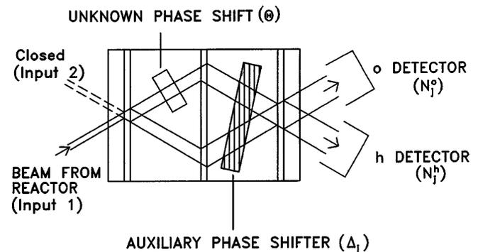
FIG. 1. Scheme of a perfect crystal neutron interferometer of the Mach-Zehnder type.
